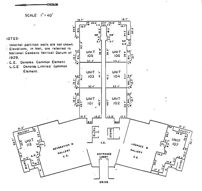
l<sup>st</sup> floar contains 8 apartment units having the following limiting elevations. Lower limits of units = Elev<u>15.83'</u> Upper limits of units = Elev<u>23.95'</u>
