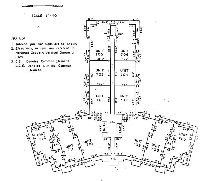
7<sup>th</sup> floor contains 12 apartment units having the following limiting elevations Lower limits of units = Elev. <u>72.00'</u> Upper limits of units = Elev. <u>80.12'</u>
