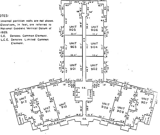
9<sup>th</sup> floor contains 12 apartment units having the following limiting elevations Lower limits of units = Elev. 89.66' Upper limits of units = Elev 97.78
