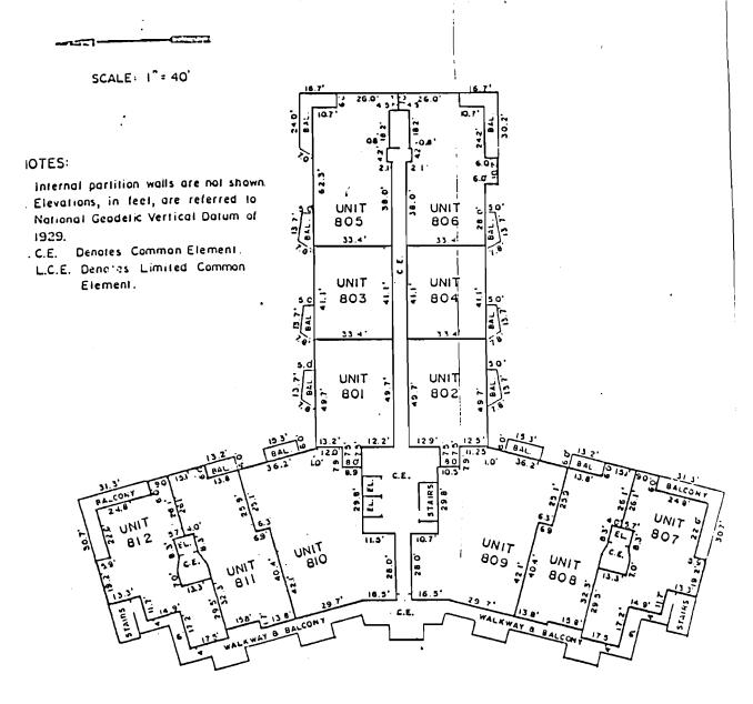
8<sup>th</sup> floor contains 12 apartment units having the following limiting elevations Lower limits of units = Elev. 80.83' Upper limits of units = Elev. 88.95'
