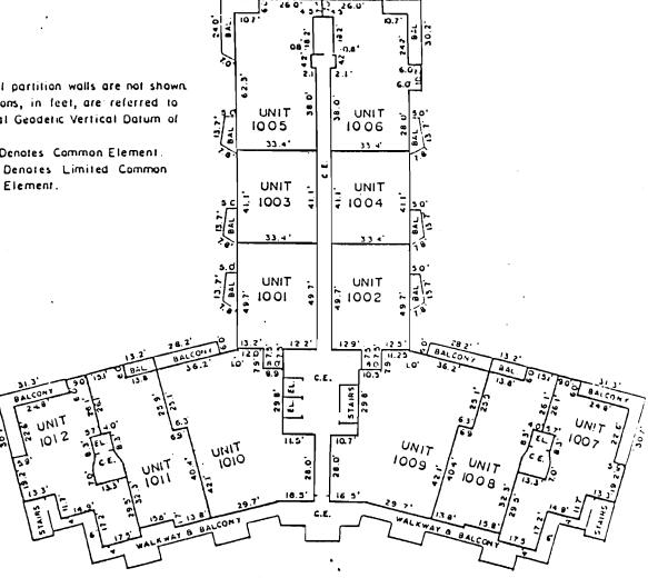
10<sup>th</sup> floor contains 12 apartment units having the following limiting elevations 98.50' Lower limits of units = Elev. Upper limits of units = Elev. 106.62
