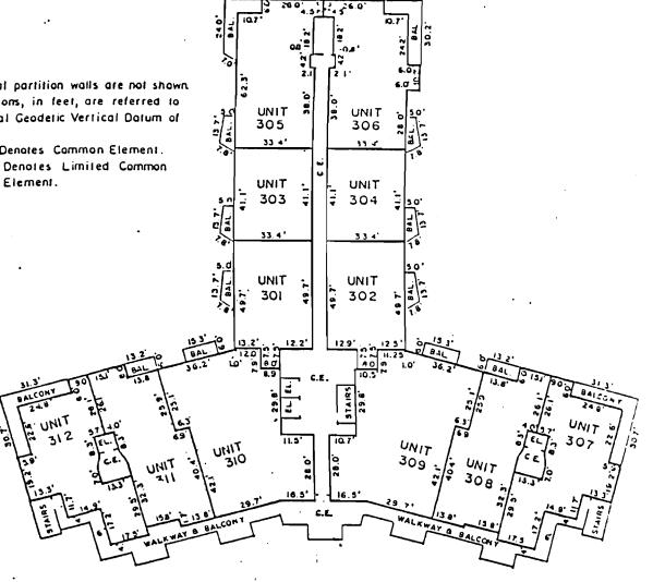
3<sup>rd</sup> floor contains 12 apartment units having the following limiting elevations 36.66 Lower limits of units = Elev. 44.77 Upper limits of units = Elev.
