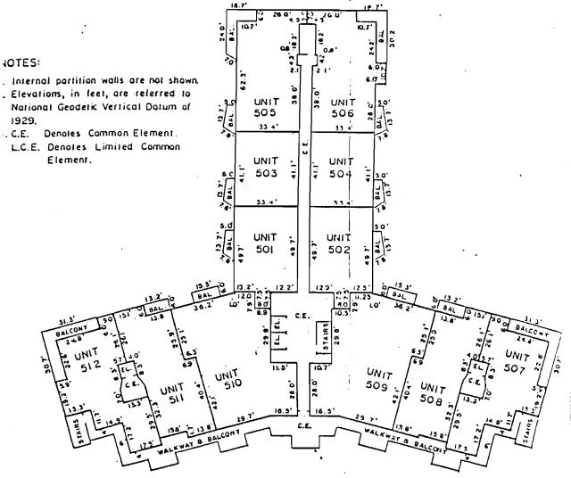
5<sup>th</sup> floor contains 12 apartment units having the following limiting elevations , Lower limits of units = Elev. 54.33 Upper limits of units = Eley 62.45
