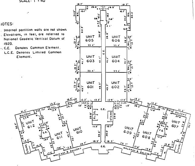
6<sup>th</sup> floor contains 12 apartment units having the following limiting elevations Lower limits of units = Elev. 63.16' Upper limits of units = Elev. 71.28'
