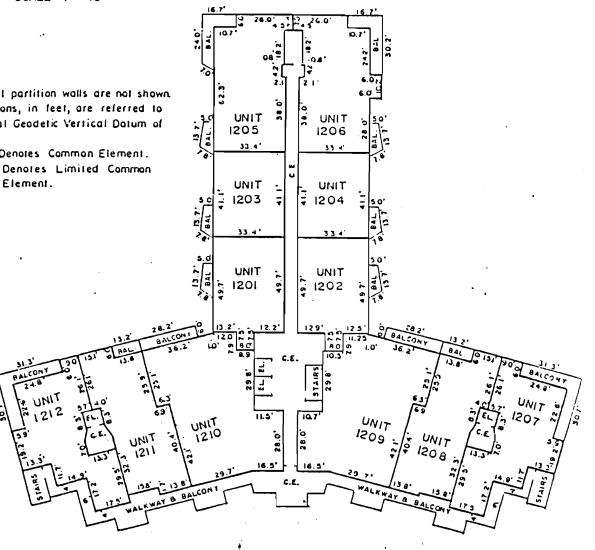
12<sup>1h</sup> floor contains 12 apartment units having the following limiting elevations 116.16 Lower limits of units = Elev.\_ 124.28 Upper limits of units = Elev\_
