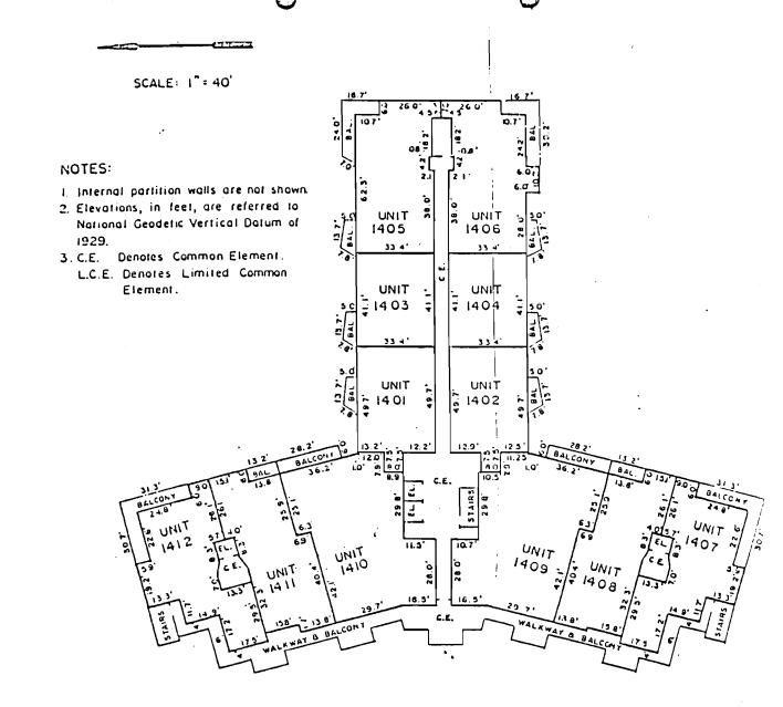
14<sup>th</sup> floor contains 12 apartment units having the following limiting elevations - Lower limits of units = Elev. <u>133.83'</u> Upper limits of units = Elev. <u>141.95'</u>
