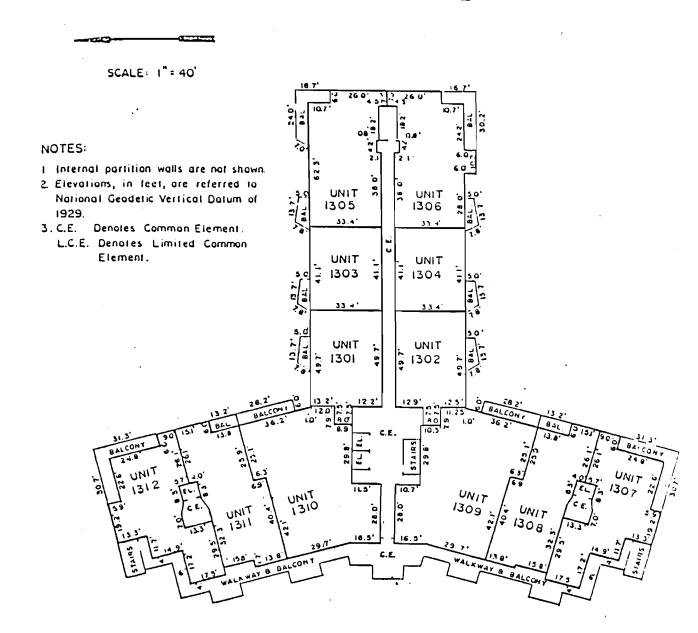
13<sup>th</sup> floor contains 12 apartment units having the following limiting elevations Lower limits of units = Elev. 125.00' Upper limits of units = Elev. 133.12'
