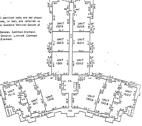
15<sup>th</sup> floor contains 12 apartment units having the following limiting elevations Lower limits of units = Elev. 142.66 Upper limits of units = Elev 150.78
